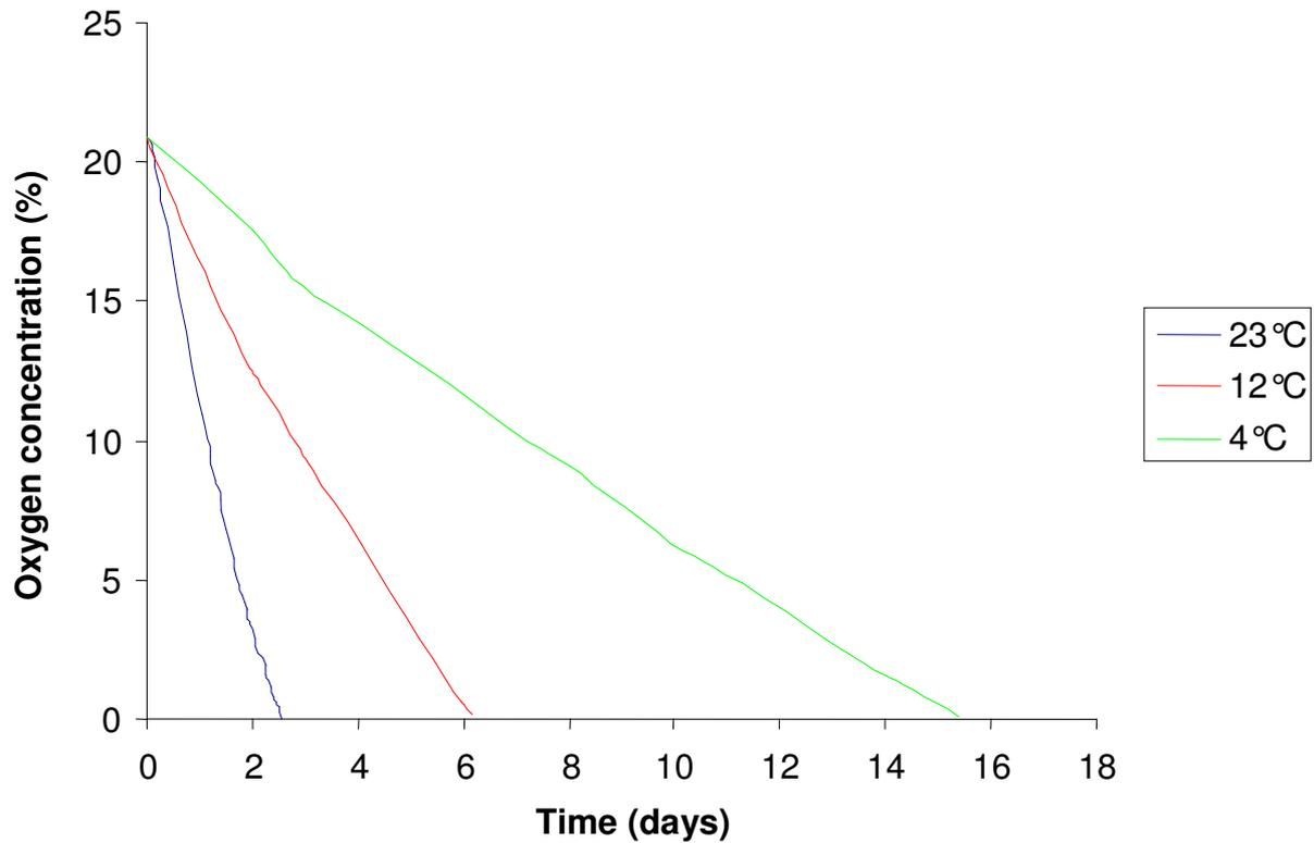
The above curve shows the oxygen consumption of 120 grams of rocket by respiring in a 5 litre container. The measurements were taken at 4 °C, 12 °C and 23 °C, respectively. The curves show how important temperature is to respiration.
