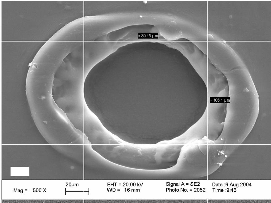
The ultimate solution for perforation plastic film is with a laser, but it is also the most expensive of the existing solutions, as it requires expensive specialist equipment. It is possible to make holes down to approx. 10 μm thicknesses and up to 200 μm. Laser perforation will typically make slightly oval holes. The advantage of laser perforation is that it is proportionately easy to control the size of the hole.
